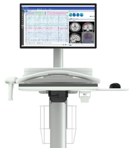
Figure 2: An image of the BrainView NeuralScan System developed by Medeia Inc. The BrainView system is portable, easy-to-use, and non-invasive. The BrainView system is a 21-channel EEG/ERP amplifier with a dedicated laptop and testing supplies. The system utilizes high-quality circuit boards and components to allow for high-quality brain measurements, as well as essential heart rate variability data.
