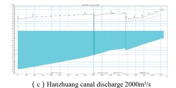
Figure 6. Simulated water surface of Taogou River - Xingou River - Beiluo Catchwater Drain under different flow conditions in Hanzhuang Canal
