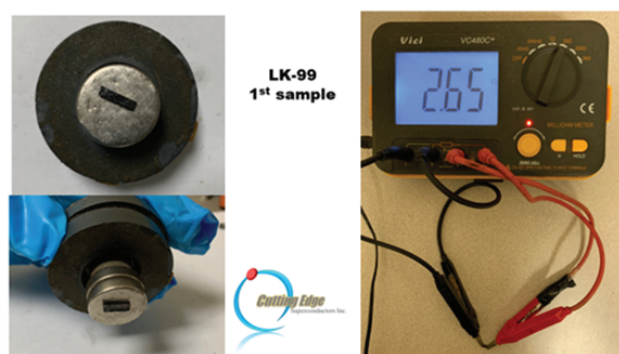
Figure 4. LK-99 sample made by solid-state reaction, according to the recipe from the Korean company [1,2]. Note that it shows the ferromagnetic attraction to the magnet and metallic behavior with resistance 2.65 ohm.
