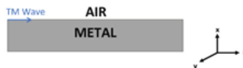
Figure 1. Plasmonic wave propagating along the boundary of two materials.
