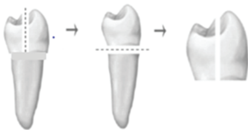
Figure 5. Sectioning of the tooth longitudinally in a mesiodistal direction
