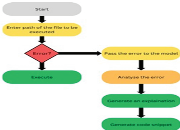
fig1. AI Based Code Error Explainer overview
