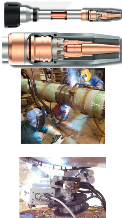
Figure 7. A view of robotized GMA welding torch with cooling system of 9°- Long duration tip system COLD Tip and automatic bug GMA girth welding of pipeline butt joints in fixed PG (5G) position [3, 12]
